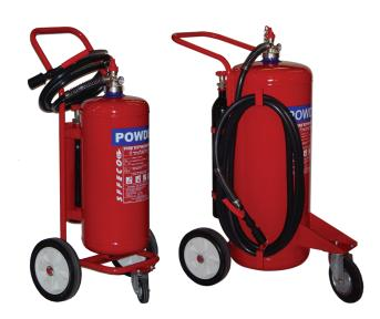
SFFECO Mobile Dry Powder Fire Extinguishers with External CO2 Cartridge are fired in two stages. Turning the rotary valve on CO2 cartridge releases the CO2 into the cylinder filled with powder and the cylinder is filled with compressed aerated powder. This compressed aerated powder is released by pressing the control lever at the nozzle and directing at the fire.
