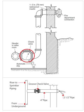
**① Note.** These valves can be installed horizontally (clapper hanging in upper position) or vertically (with flow in upward direction). Flow direction indicated by the arrow on the body must always be considered.
